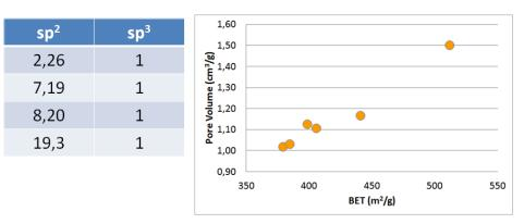
sp<sup>2</sup>/sp<sup>3</sup> ratio and Pore volume vs BET for some of the RGO prepared
